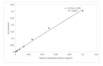
Figure 1. Standard curve of Ti
